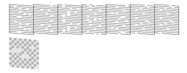
If you don't see any improvement after cleaning the print head three or four times, check the solutions beginning on page 96. You can also turn the printer off and wait overnight—this allows any dried ink to soften—and then clean the print head again.
